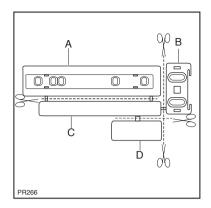
Place guide (A) on the inside part of the furniture door, in the upper and lower positions as shown in the figure and mark the position of external holes. After having drilled holes, fix the guide with the screws supplied.
